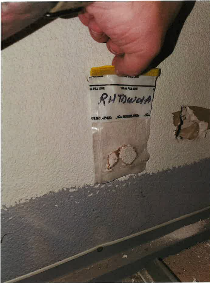
Photo 2: View of the bulk sample collected from the textured drywall in the east main entry to the building. No asbestos was identified to be present in the texture, drywall mud or sheet rock.
