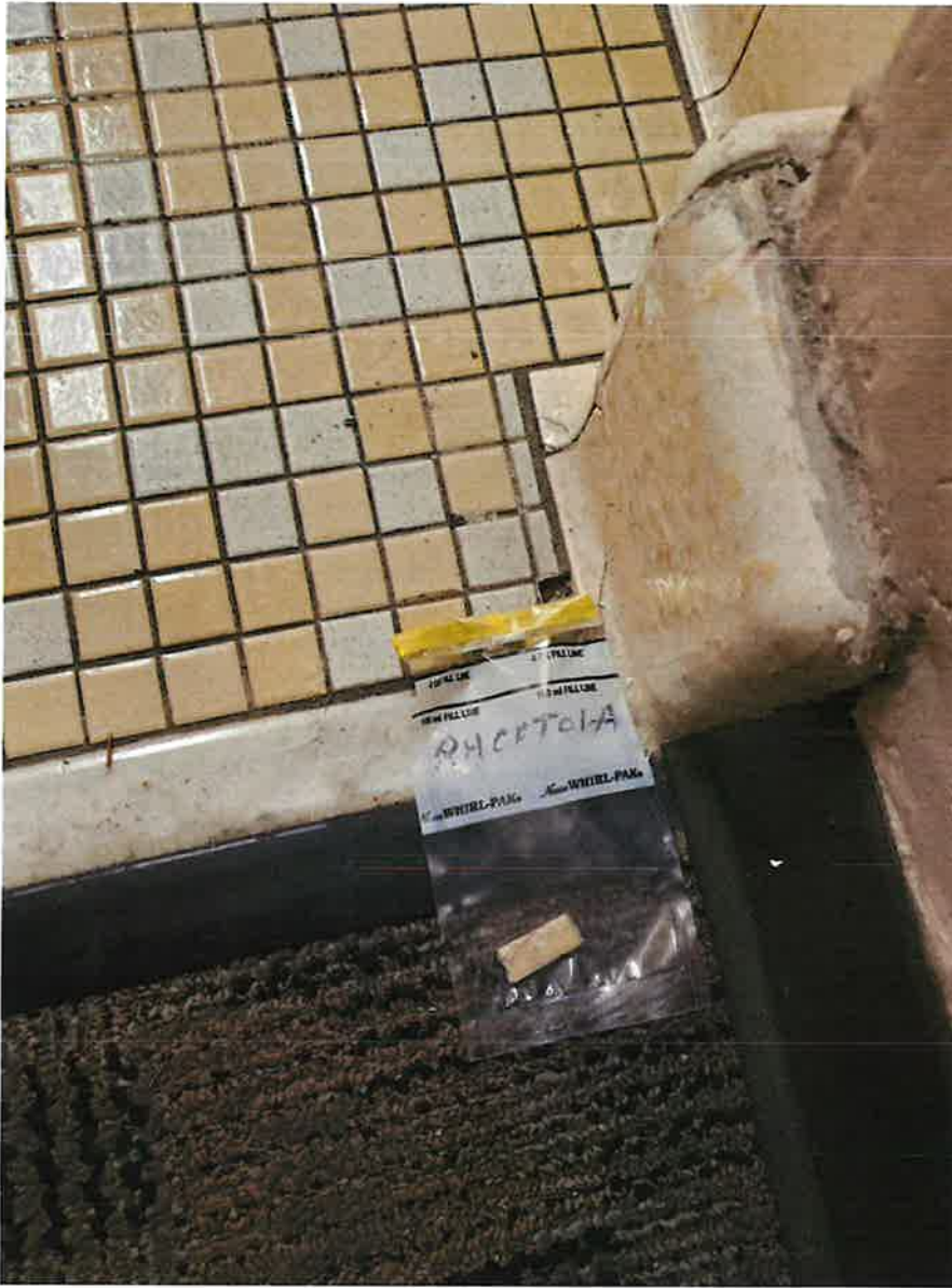
Photo 1: View of the bulk sample collected from the ceramic floor tile and mortar in the men restroom. No asbestos was identified to be present in the ceramic tile or mortar.
